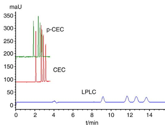
**Fig. 4.** Electropherograms of four compounds using the prepared column in the modes of p-CEC, CEC and LPLC. Experimental condition: Capillary length 33 cm (24.5 cm)  $\times$  100  $\mu$ m, other experimental conditions and peak identification are the same as in Fig. 3.
