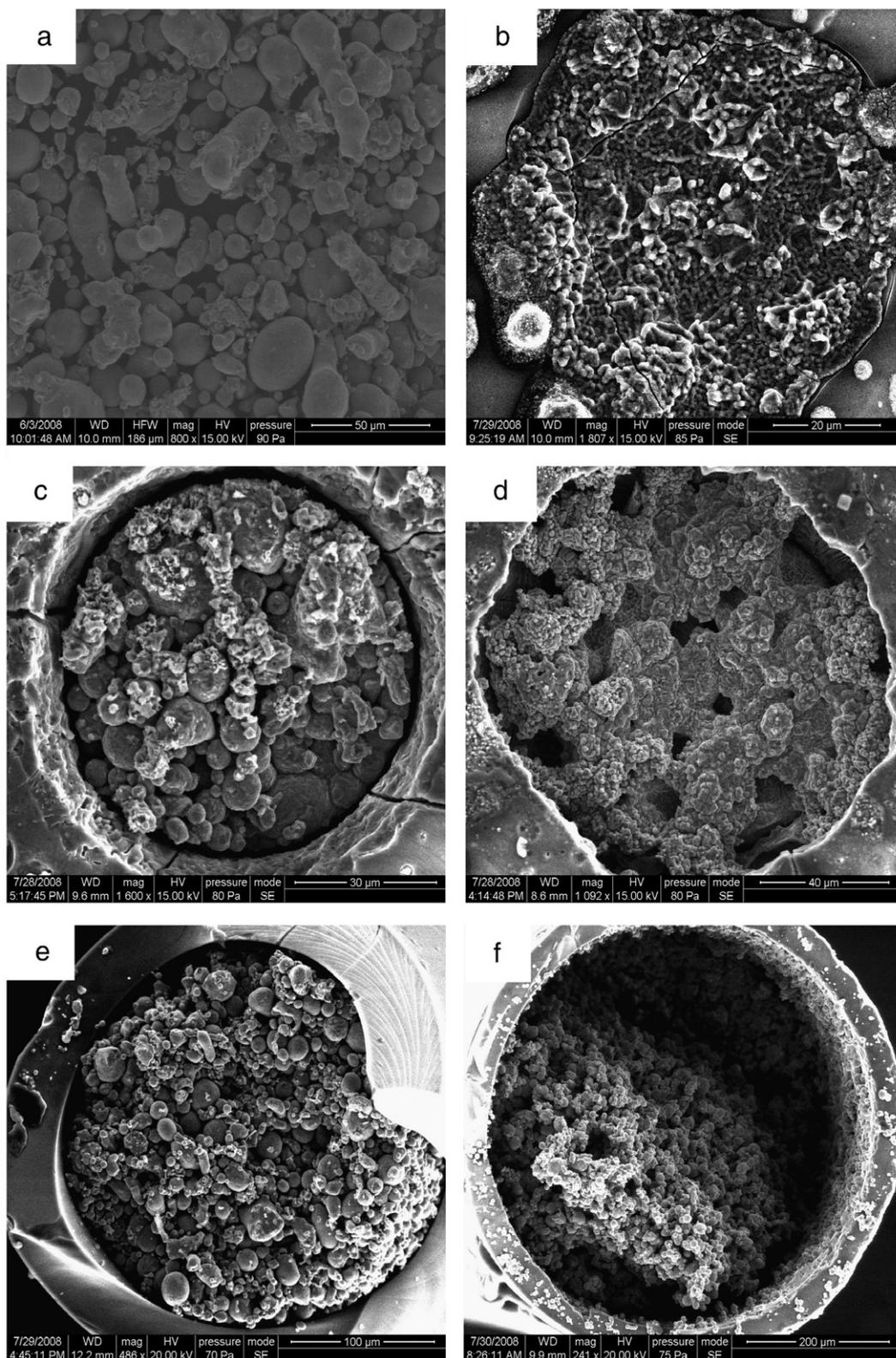
**Fig. 1.** SEM image of stainless steel particles and frits sintered about 20 s in different i.d. capillary tubes. a: tapped steel particles at the tip of the capillary, b–f: the sintered SS particles in the capillaries with inner diameters 50, 75, 100, 250 and 530 µm, respectively.
