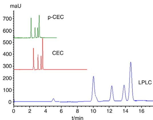
**Fig. 3.** Electropherograms of the four compounds using the prepared column in the modes of p-CEC, CEC and LPLC. Experimental condition: Capillary length 33 cm (24.5 cm)  $\times$  75  $\mu$ m, packing length = 16.5 cm; injection: 10 kV  $\times$  5 s; 20  $^{\circ}$ C, 200 nm, buffer: ACN/10 mMTris = 9:1 (v/v); pH = 8.5. p-CEC 30 kV + 12 bar (inlet); CEC: 30 kV + 12 bar (both end); LPLC: 12 bar (inlet). Peak order: 1. thiourea, 2. benzene, 3. toluene, and 4. ethylbenzene.
