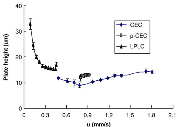
Fig. 5. Plate height of ethylbenzene as a function of migration velocity on column B in the modes of p-CEC, CEC and LPLC. Experimental conditions are the same as in Fig. 4.
