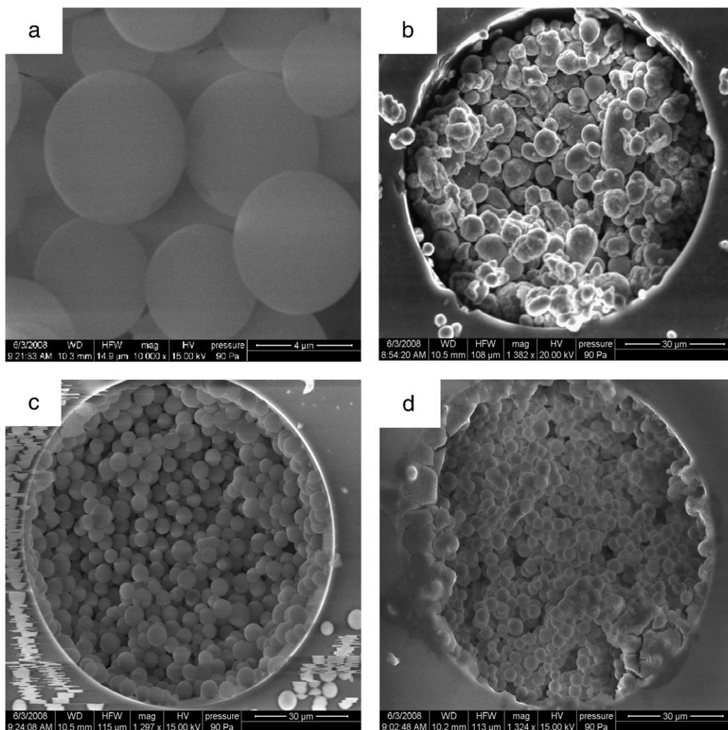
**Fig. 2.** SEM image of the stationary phase particles and the packed capillary column at different cross sections. a. the stationary phase particles, b. the cross section of sintered inlet frit, c. the cross section of stationary phase, and d. the cross section of outlet frit.
