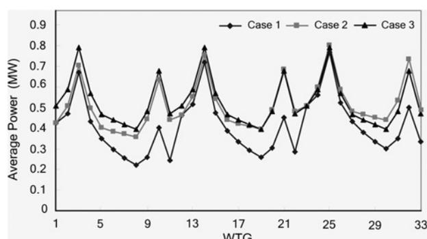
Fig. 12 Average power curves of WTGs for the three cases
