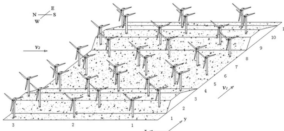
Fig. 11 Optimal wind farm layout
