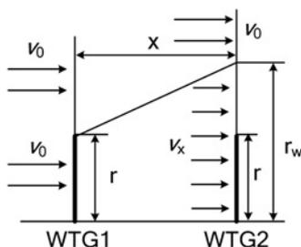
Fig. 4 Wake effect representation of two WTGs in a flat land
