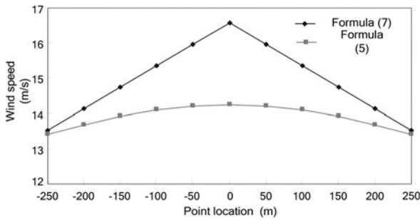
Fig. 3 Wind speed curves over a hill
