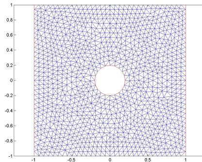
Figure 4.6: A triangular mesh on a square domain with a circular hole
