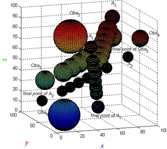
Fig. 12. Planned paths of  $A_1$ ,  $A_2$ ,  $A_3$  and movement of obstacle 3 in three dimensions with obstacles.
