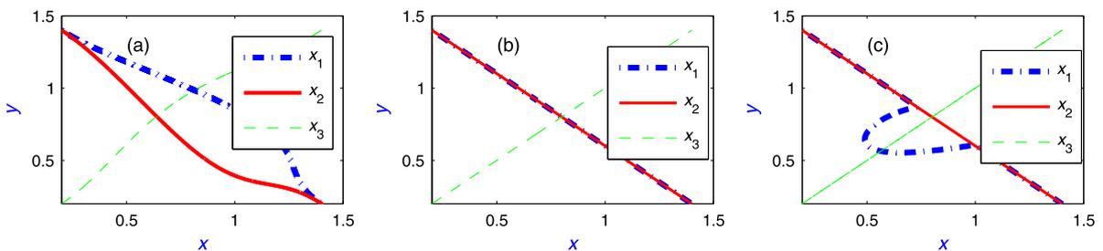
Fig. 8. Planned paths of  $A_1$ ,  $A_2$  and  $A_3$  under environment in [10]. (a) are paths given in [10]. (b) and (c) are paths without or with conflict resolution, respectively.
