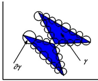
Fig. 1. Obstacle  $k$  and its boundary, that is covered with circles.
