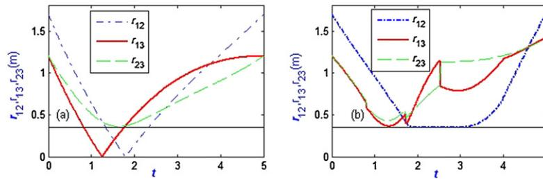
Fig. 9. Distances between any two mobile objects \$A\_1, A\_2\$ and \$A\_3\$. (a) and (b) without or with priority scheme and conflict resolution respectively.
