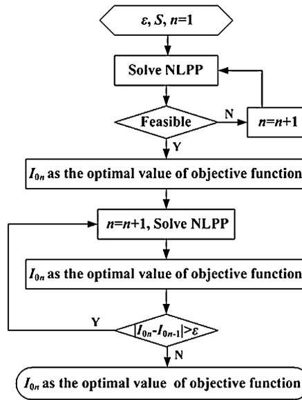
Fig. 2. Algorithm for solving the NLPPs.
