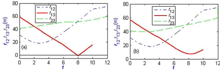
Fig. 6. Distances between any two mobile objects  $A_1$ ,  $A_2$  and  $A_3$ . (a) and (b) without or with priority scheme and conflict resolution respectively.
