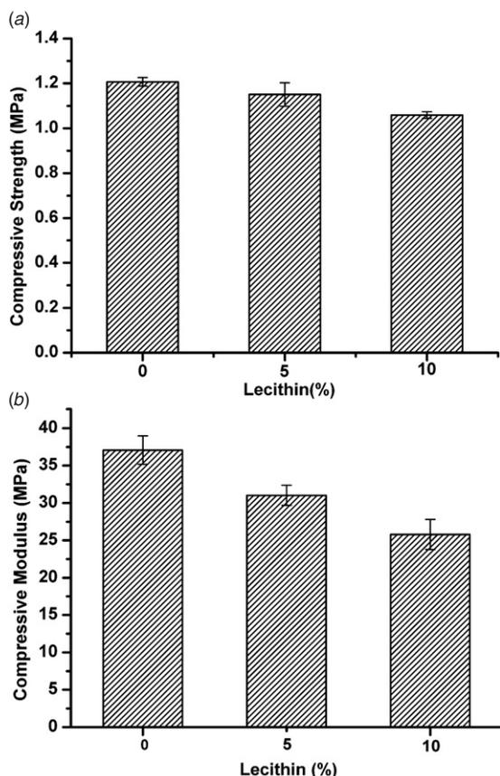
**Figure 3.** The compressive property testing results of the scaffolds. (a) The compressive strength value of 0%L, 5%L and 10%L scaffolds and (b) the compressive modulus of 0%L, 5%L and 10%L scaffolds.
