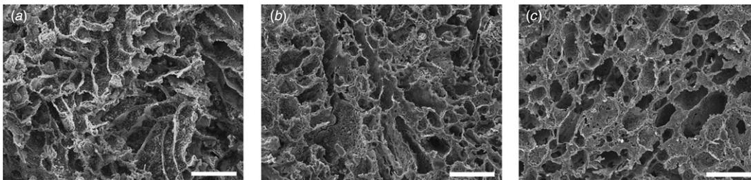
**Figure 1.** SEM morphology of interconnected porous structure of scaffolds. (a) 0%L scaffold, (b) 5%L scaffold and (c) 10%L scaffold. Scale bar is 200  $\mu\text{m}$ .
