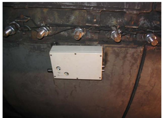
Fig. 3. Installation image for the wireless transmitter device mounted on the mill shell.
