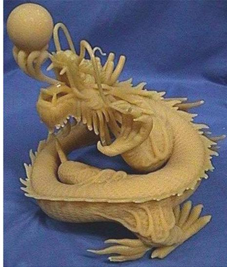
**Figure 4.** A HIPS/epoxy SLS part with complicated structures.
