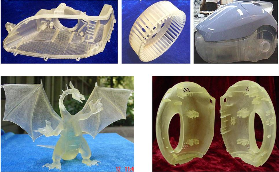
**Figure 11.** SLA parts made from the free radical-cationic hybrid photopolymer with complicated structures.
