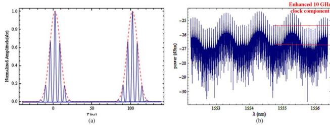
Fig. 1. Simulated waveform and spectrum of 160-Gb/s signal after EAM1. (a) Waveform; (b) spectrum.
