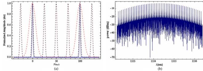
Fig. 2. Simulated waveform and spectrum of 160-Gb/s signal after two EAMs. (a) Waveform; (b) spectrum.
