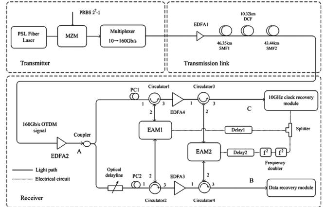
Fig. 3. Experimental setup of 160-Gb/s OTDM system. PSL: Picosecond fiber laser. MZM: Mach-Zehnder modulator. PC: Polarization controller. EDFA: Erbium-doped fiber amplifier.
