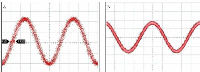
Fig. 5. Waveform of the 10-GHz extracted clock from 160-Gb/s OTDM.
