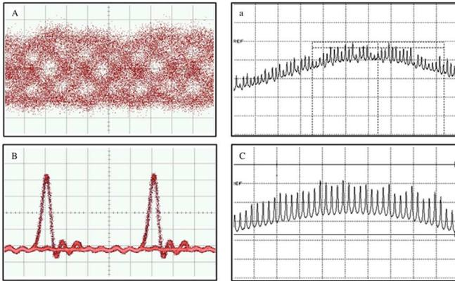
Fig. 4. Eye diagrams of the positions at A, B, C in setup. (A) Eye diagrams of 160-Gb/s signal at receiver part. (a) Spectrum of 160-Gb/s signal. (B) Eye diagrams of demultiplexed 10 Gb/s from 160 Gb/s. (C) Spectrum of enhanced 10-GHz clock after EAMs.
