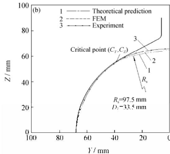
**Fig. 10. Predicted and experimental surface profiles of the outgoing workpiece: (a) oval pass; (b) round pass.**
