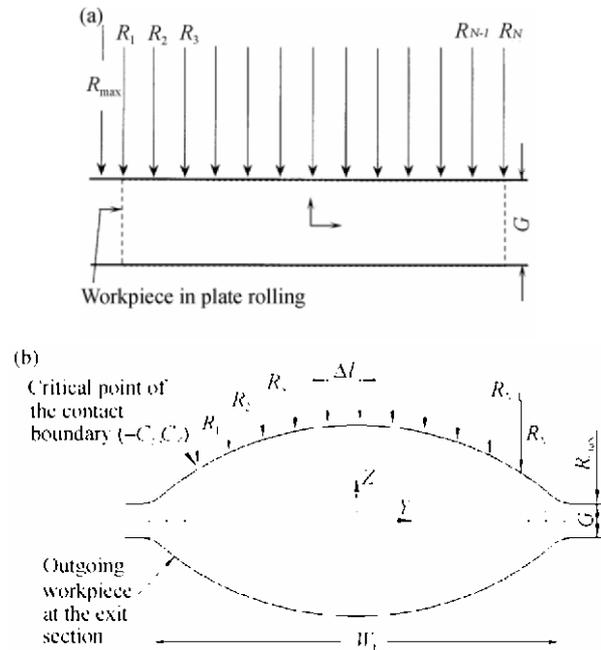
Fig. 5. Discrete distribution of radius at the exit section: (a) in strip or plate rolling; (b) in rod or bar rolling
