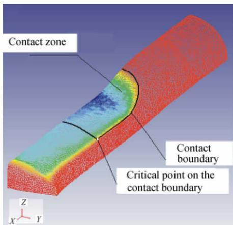
**Fig. 8. Contact boundary and contact zone in oval pass rolling.**
