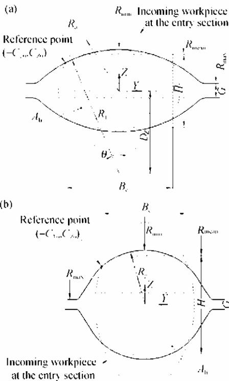
Fig. 4. Parameter signification for the calculation of mean roll radius by Satio *et al.*'s model [2]: (a) oval pass; (b) round pass.
