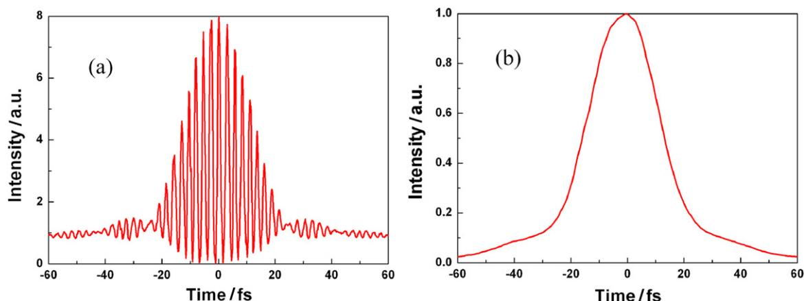
**Figure 7.** Measured autocorrelation traces. (a) Interferometric autocorrelation and (b) intensity autocorrelation.
