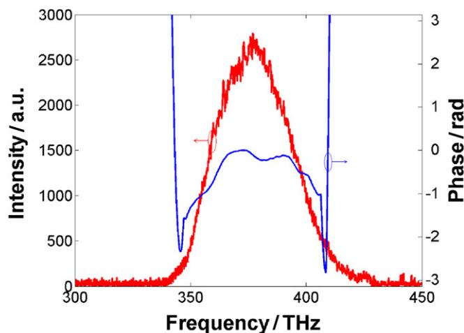
**Figure 4.** Measured spectrum and the retrieved spectral phase.
