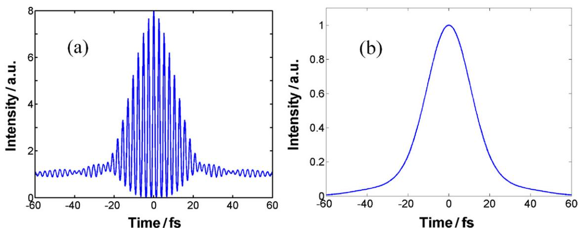
**Figure 6.** Simulated autocorrelation traces with reconstructed pulsed electric field. (a) Interferometric autocorrelation and (b) intensity autocorrelation.
