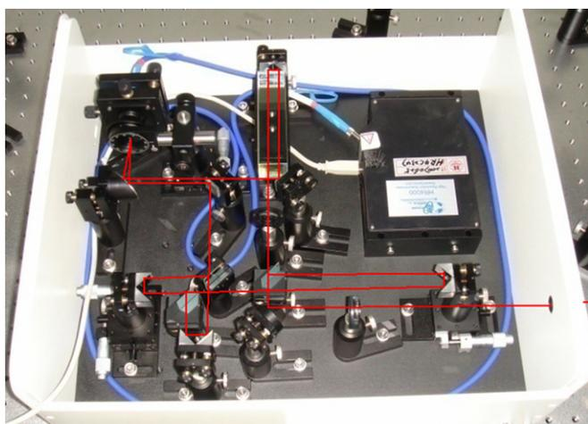
**Figure 1.** Our home-made SPIDER setup and the optical path.
