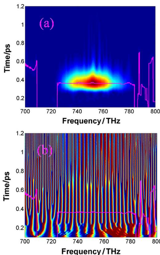
**Figure 3.** Wavelet transform of the spectral interferogram. (a) Intensity topography and (b) phase topography. The ridge of the wavelet transform is indicated with a pink coloured line.
