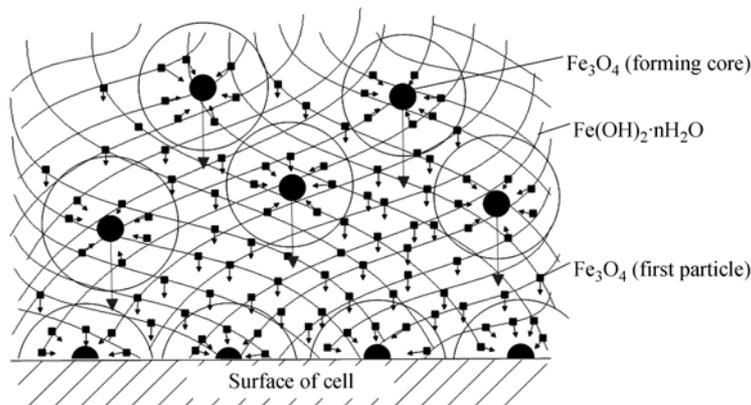
**Figure 6** Sketch of how microorganism cells are coated with  $\text{Fe}_3\text{O}_4$  layers.
