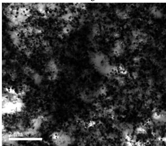
Figure 5 SEM photo of Fe<sub>3</sub>O<sub>4</sub> particles fabricated by sol-gel method.
