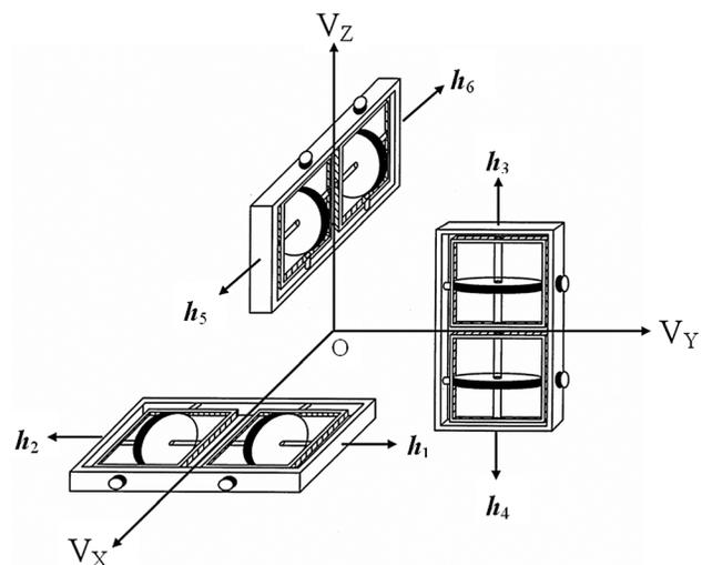
Fig. 2 Configuration of three orthogonally mounted scissored pairs of CMGs
