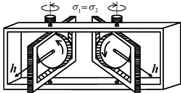
Fig. 1 Configuration of scissored pair of CMGs
