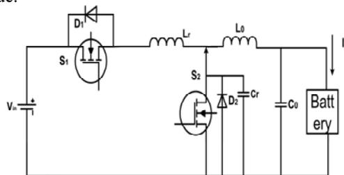
Fig. Novel converter for battery chargers
