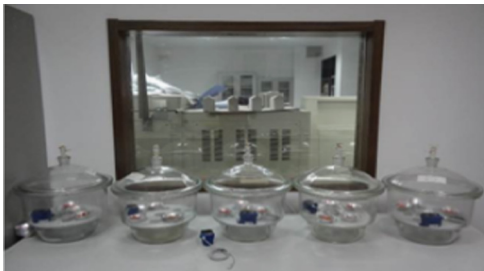
Figure 3 Experimental drying vessels and automatic temperature and humidity recorder.
