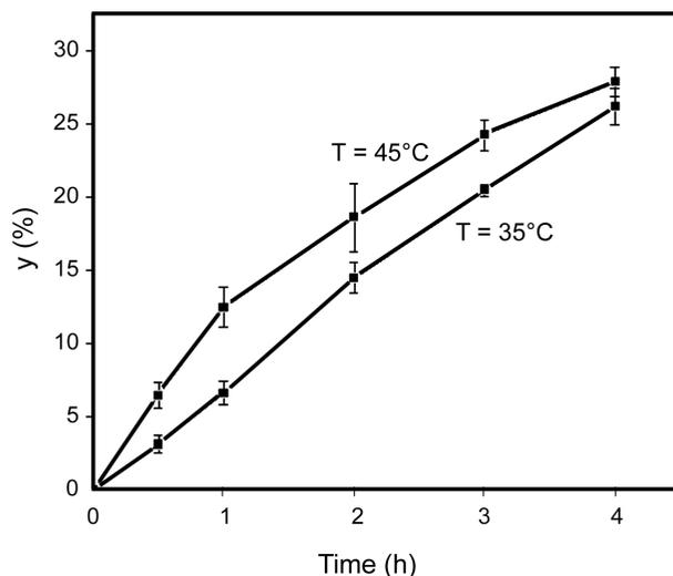
**Figure 8.** The AMP release curves at different temperatures.
