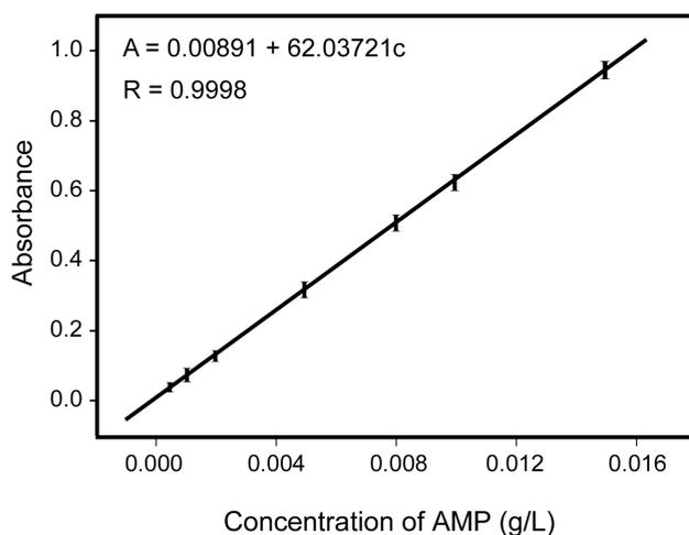
**Figure 3.** The calibration curve of AMP aqueous solutions.
