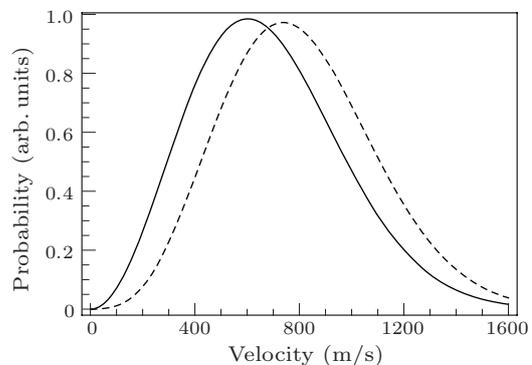
**Fig. 3.** Atomic velocity distribution curves in the calcium atomic beam, the solid line represents velocity distribution in the hot oven, the dashed line indicates velocity distribution in the thermal beam outside the oven. Here  $m = 6.6 \times 10^{-26}$  kg,  $T = 873$  K.
