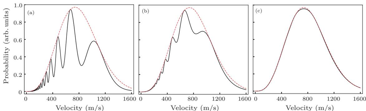
**Fig. 5.** Population inversion for the atomic beam crossing a distance  $z$  from the laser waist. The laser waist  $w_0 = 0.2$  mm, the laser power is  $P = 10$  mW, distance  $z$ : (a)  $z = 0.1$  m, (b)  $z = 0.2$  m, (c)  $z = 0.5$  m. The total probabilities are (a) 67%, (b) 86%, (c) 99%, respectively.
