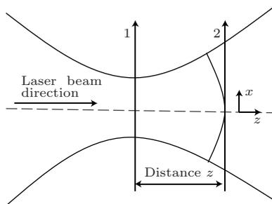
**Fig. 1.** The laser beam and two atomic trajectories, (1) resulting in Rabi oscillations, (2) resulting in an adiabatic passage.
