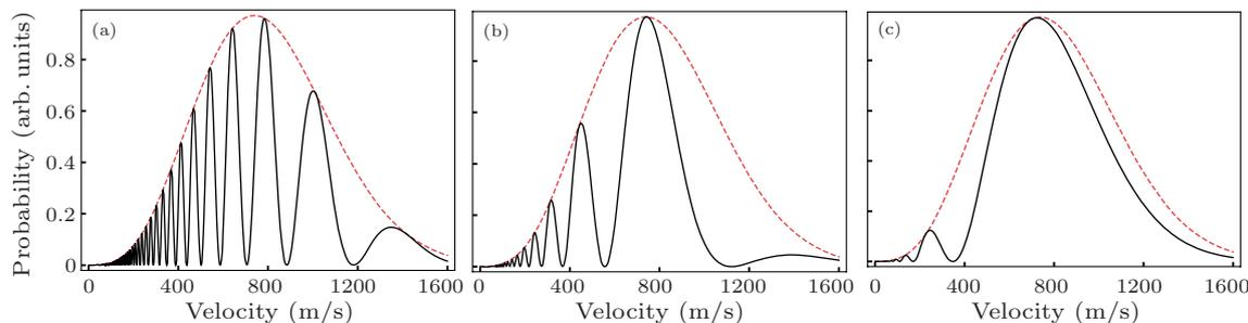
**Fig. 4.** Population inversion for the atomic beam after crossing the laser waist; the dashed line represents the velocity distribution, the solid line indicates the probability that corresponds to the velocity at which atoms are pumped to the upper level. The laser waist  $w_0 = 1$  mm, the laser power is (a)  $P = 40$  mW (b)  $P = 4$  mW (c)  $P = 0.4$  mW, the total probability is (a) 50% (b) 46% (c) 76%, respectively.
