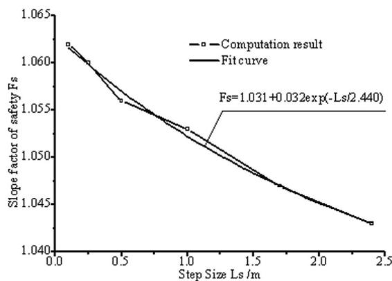
**Figure 7** Influence of the step size  $L_s$  on the slope factor of safety  $F_s$  in Example 1
