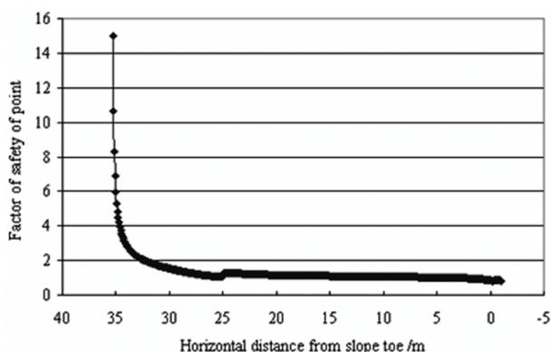
**Figure 11** Distribution of factor of safety of point on the critical slide surface in Example 3
