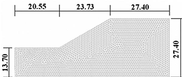
Figure 3 Finite element model of slope in Example 1
