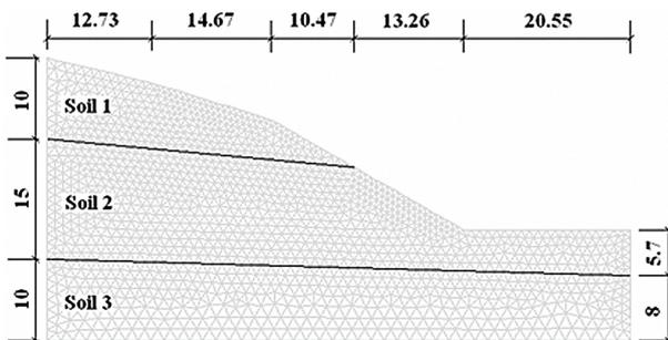
**Figure 8** Finite element model of slope in Example 3
