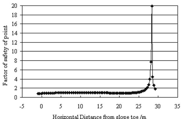
**Figure 6** Distribution of factor of safety of point on the critical slip surface in Example 1
