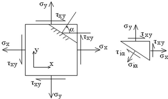
**Figure 1** Stress state of unit body in slope
