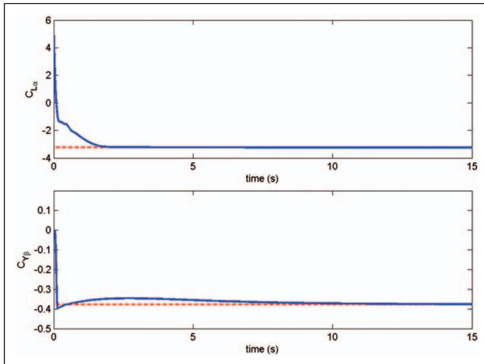
Figure 5. Time histories of the estimation for the aerodynamic force coefficients.
