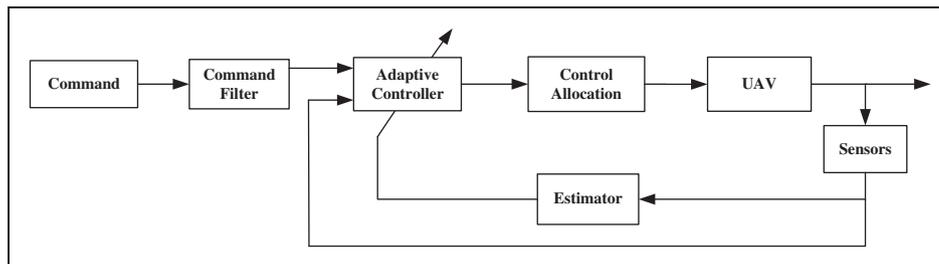
Figure 1. Framework of the flight control system.
