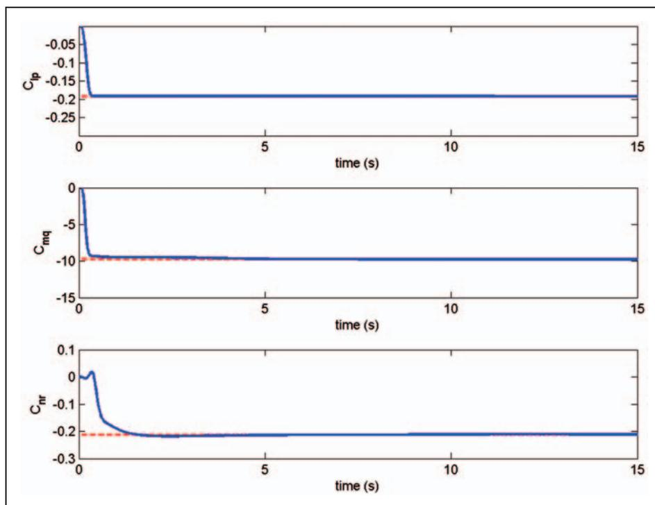
Figure 6. Time histories of the estimation for the aerodynamic moment coefficients.
