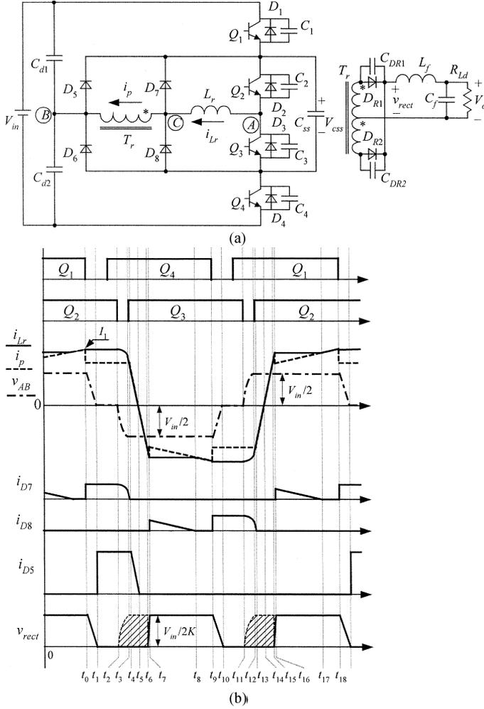
Fig. 1. The original ZVS PWM TL converter. (a) Main circuit. (b) Key waveforms.
