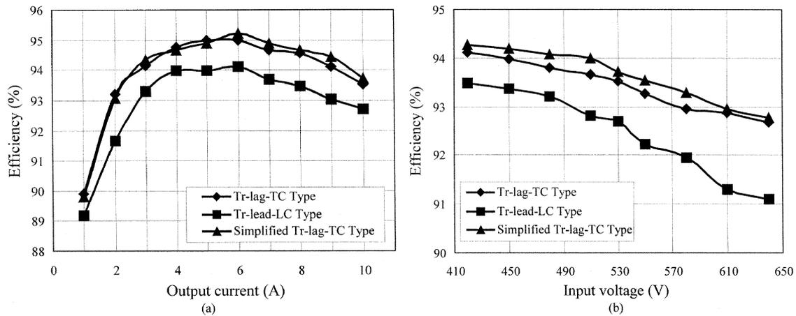
Fig. 12. The overall efficiency. (a) Efficiency at different output current under the normal input voltage. (b) Efficiency at full load under different input voltage.
