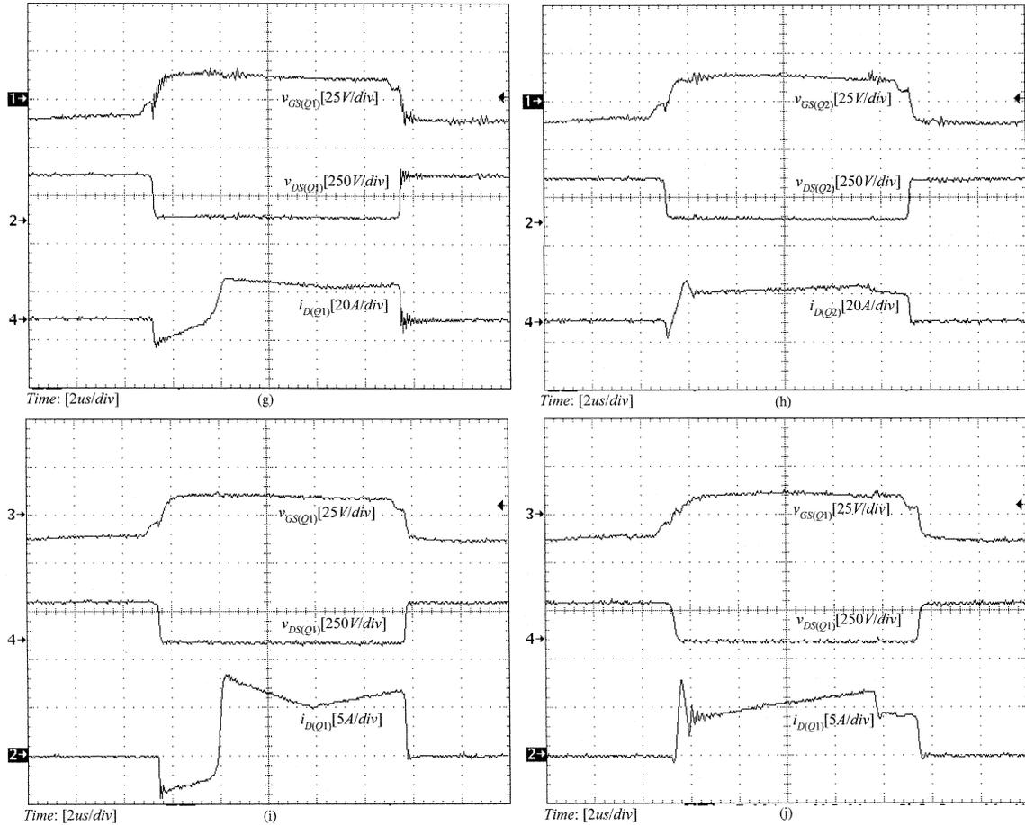
Fig. 11. (Continued.) Experimental waveforms. (g)  $v_{GS}$ ,  $v_{DS}$ , and  $i_D$  of the leading switch  $Q_1$  under full load. (h)  $v_{GS}$ ,  $v_{DS}$ , and  $i_D$  of the lagging switch  $Q_2$  under full load. (i)  $v_{GS}$ ,  $v_{DS}$ , and  $i_D$  of the leading switch  $Q_1$  under 20% full load. (j)  $v_{GS}$ ,  $v_{DS}$ , and  $i_D$  of the lagging switch  $Q_2$  under 20% full load.
