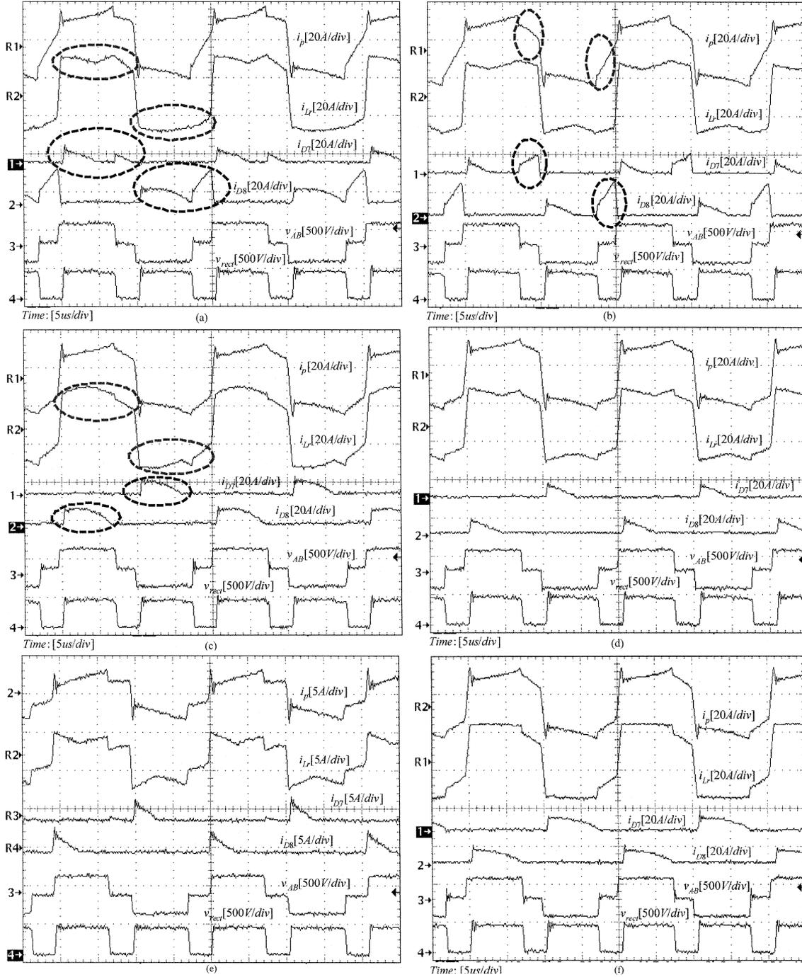
Fig. 11. Experimental waveforms. (a)  $T_r$ -lead-LC Type. (b)  $T_r$ -lead-TC Type. (c)  $T_r$ -lag-LC Type. (d)  $T_r$ -lag-TC Type. (e) The waveforms of  $T_r$ -lag-TC Type under 10% load. (f) The waveforms of simplified  $T_r$ -lag-TC Type.
