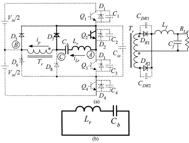
Fig. 8. Equivalent circuit of  $T_r$ -lead-LC Type when the clamping diodes conduct. (a) Equivalent circuit. (b) Further equivalent circuit.
