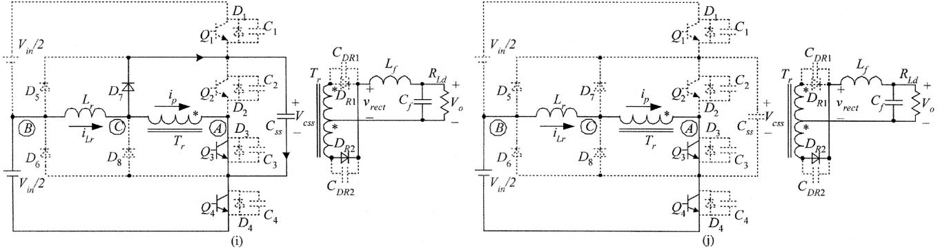
Fig. 3. (Continued.) The equivalent circuits of each switching mode. (i)  $[t_7, t_8]$ . (j)  $[t_8, t_9]$ .
