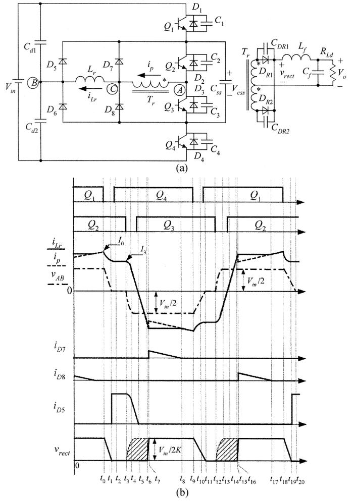
Fig. 2. The improved ZVS PWM TL converter. (a) Main circuit. (b) Key waveforms.
