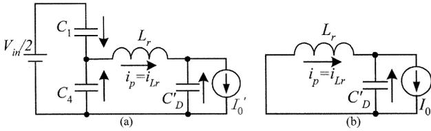
Fig. 4. Further simplified equivalent circuit of mode 1 and mode 2. (a) Mode 1. (b) Mode 2.
