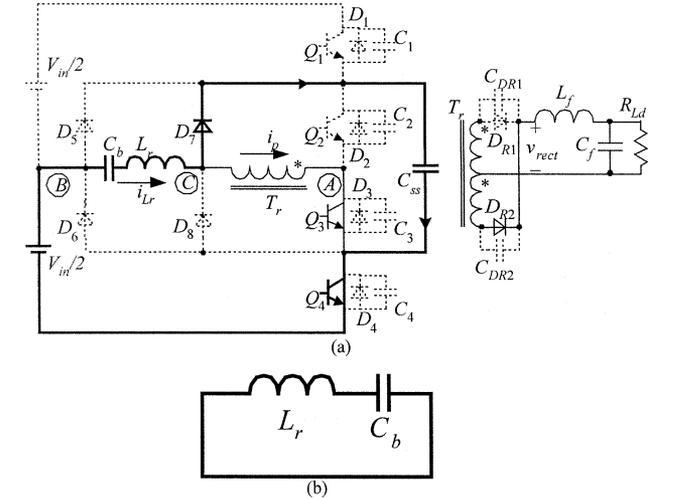
Fig. 10. Equivalent circuit of  $T_r$ -lag-LC Type when the clamping diodes conduct. (a) Equivalent circuit. (b) Further equivalent circuit.
