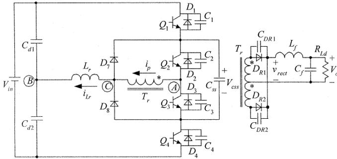
Fig. 5. Simplified improved ZVS PWM TL converter.
