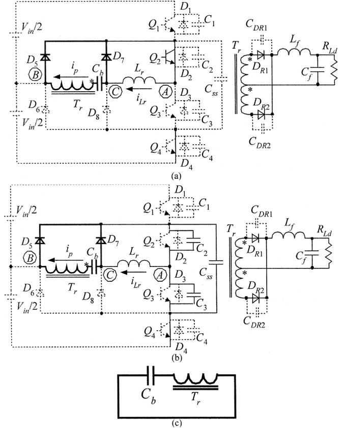
Fig. 9. Equivalent circuit of  $T_r$ -lead-TC Type when the clamping diodes conduct. (a) Equivalent circuit 1. (b) Equivalent circuit 2. (c) Further equivalent circuit.
