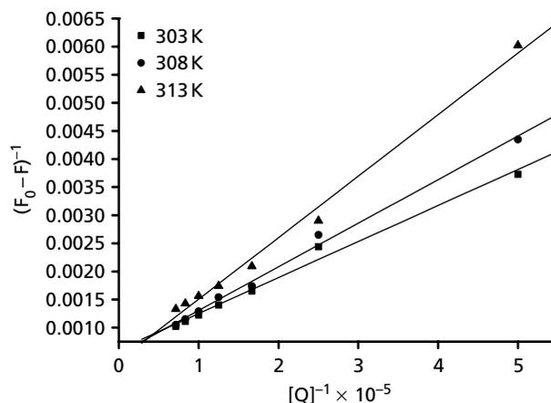
**Figure 5** Lineweaver–Burk curves of the system of Schiff base selenide–BSA at different temperatures.  $F$  and  $F_0$  are current and initial fluorescence, respectively;  $[Q]$  is ligand concentration;  $\lambda_{\text{ex}} = 282 \text{ nm}$ ,  $\lambda_{\text{em}} = 340 \text{ nm}$ ; BSA concn:  $1.0 \times 10^{-5} \text{ mol L}^{-1}$ ;  $\text{pH} = 7.4$ .
