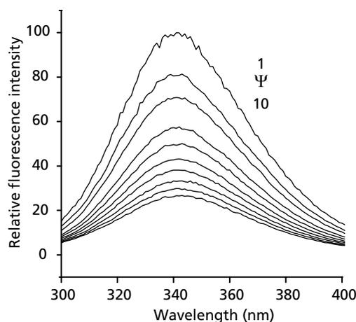
**Figure 2** The fluorescence emission spectra of Schiff base selenide–BSA system. The concn of BSA was  $1.0 \times 10^{-5}$  mol L $^{-1}$ . The molar ratio of selenide to BSA corresponded to 1–10:0, 0.2, 0.4, 0.6, 0.8, 1.0, 1.2, 1.4, 1.6, 1.8; temperature = 303 K; pH = 7.4.
