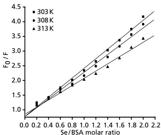
**Figure 3** Stern–Volmer curves for Schiff base selenide–BSA at different temperatures.  $F$  and  $F_0$  are current and initial fluorescence, respectively;  $\lambda_{\text{ex}} = 282 \text{ nm}$ ,  $\lambda_{\text{em}} = 340 \text{ nm}$ ; BSA concn:  $1.0 \times 10^{-5} \text{ mol L}^{-1}$ ;  $\text{pH} = 7.4$ .
