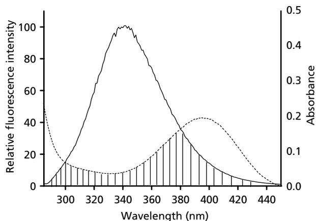
**Figure 7** The overlap of the fluorescence spectrum of BSA (real line) and the absorption spectrum of Schiff base selenide (dashed line).  $C_{\text{BSA}} = C_{\text{selenide}} = 1.0 \times 10^{-5} \text{ mol L}^{-1}$ ; pH = 7.4; temperature = 303 K.
