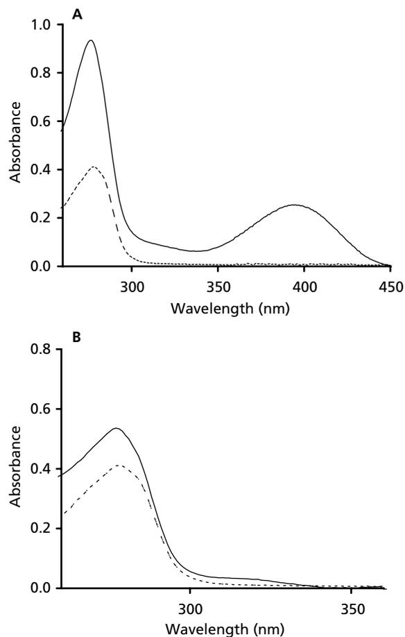
**Figure 4** Change in UV absorption spectra of BSA in the presence of Schiff base selenide (A) and differential UV absorption spectrum of complex to Schiff base selenide (solid line) (B). Dashed line represents the spectrum of BSA.  $C_{\text{BSA}} = C_{\text{selenide}} = 1.0 \times 10^{-5} \text{ mol L}^{-1}$ ;  $\text{pH} = 7.4$ ; temperature = 303 K.
