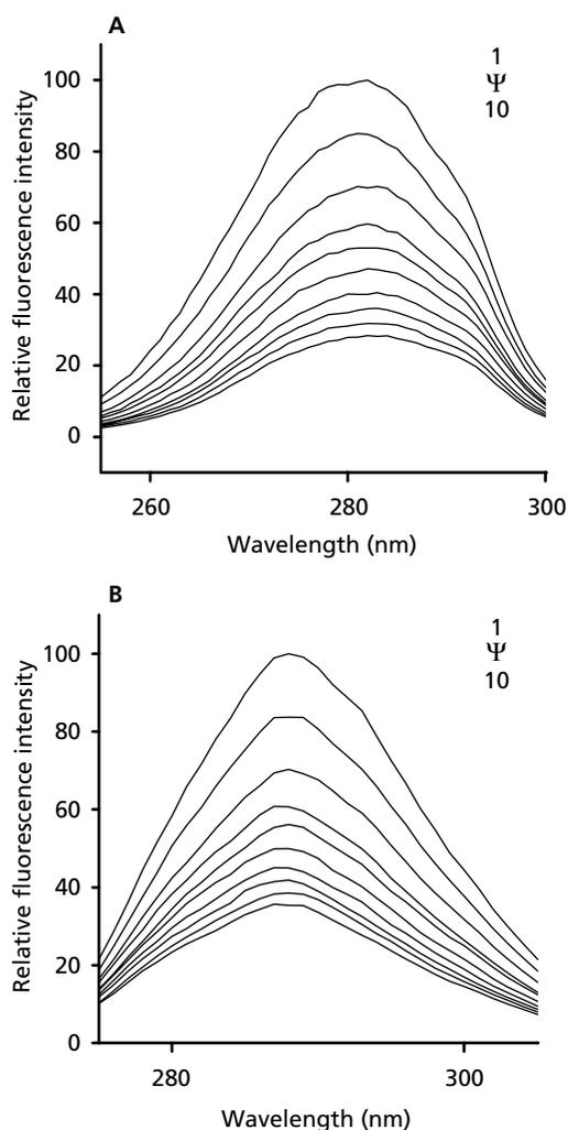
**Figure 8** The influence of Schiff base selenide on the synchronous fluorescence spectra of BSA (A:  $\Delta\lambda = 60 \text{ nm}$ ; B:  $\Delta\lambda = 15 \text{ nm}$ ). The concn of BSA was  $1.0 \times 10^{-5} \text{ mol L}^{-1}$ . The molar ratio of selenide to BSA corresponded to 1–10:0, 0.2, 0.4, 0.6, 0.8, 1.0, 1.2, 1.4, 1.6, 1.8; temperature = 303 K; pH = 7.4.
