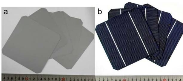
Fig. 9. (a) Silicon wafer, and (b) solar cell.
