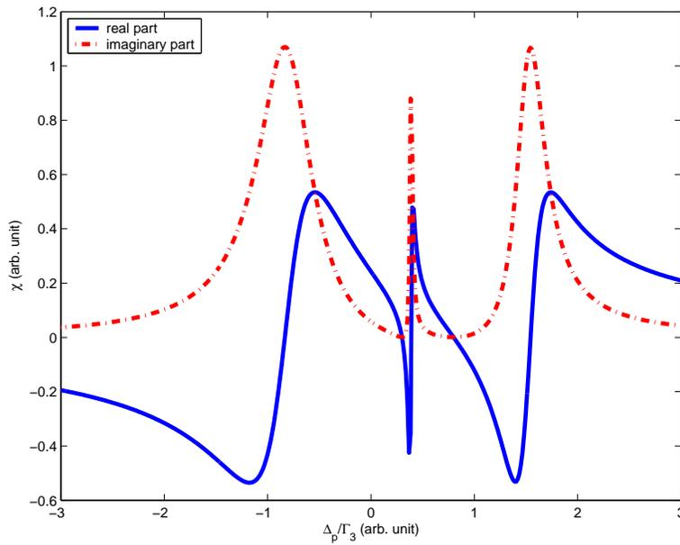
Fig. 2. The dispersive behavior of the real and imaginary parts of the electric susceptibility as the probe frequency detuning varies. Both the real and imaginary parts of  $\chi(\Delta_p)$  tend to zero at probe frequency detunings  $\Delta_p = 3.0 \times 10^7 \text{ s}^{-1}$  and  $\Delta_p = 8.0 \times 10^7 \text{ s}^{-1}$ .
