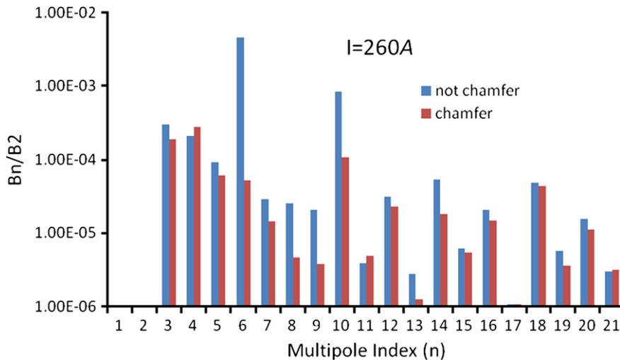
Fig. 6. High order harmonic components at current 260 A.
