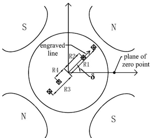
**Fig. 1.** The geometry of the harmonic coil in quadrupole magnet.
