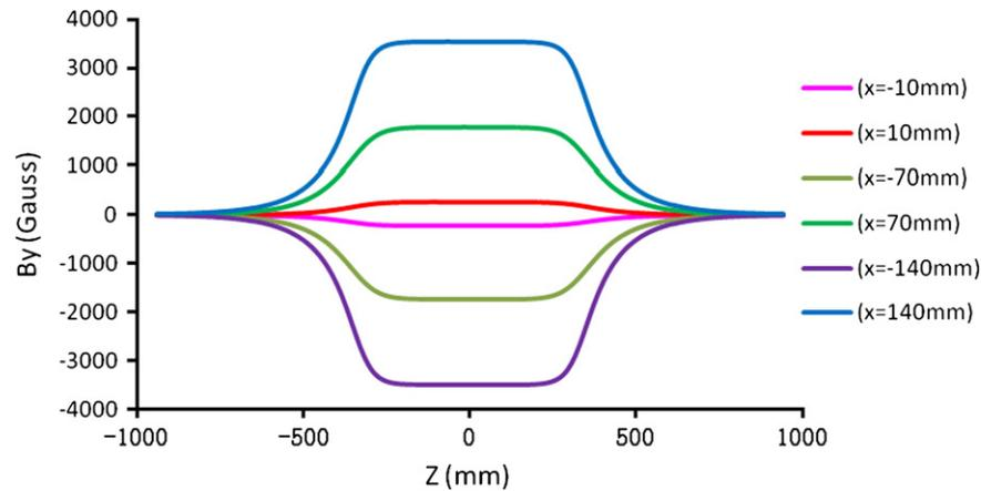
Fig. 8. Spatial distributions of the vertical component of the field  $B_y$  as function of the longitudinal coordinate  $z$ .
