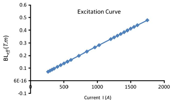
Fig. 7. Excitation curve of the magnet at the radius of 141 mm.
