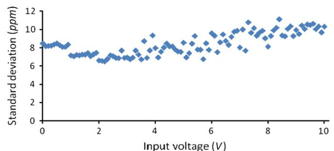
**Fig. 2.** Standard deviation of PXI-4462 device at different input standard signals.
