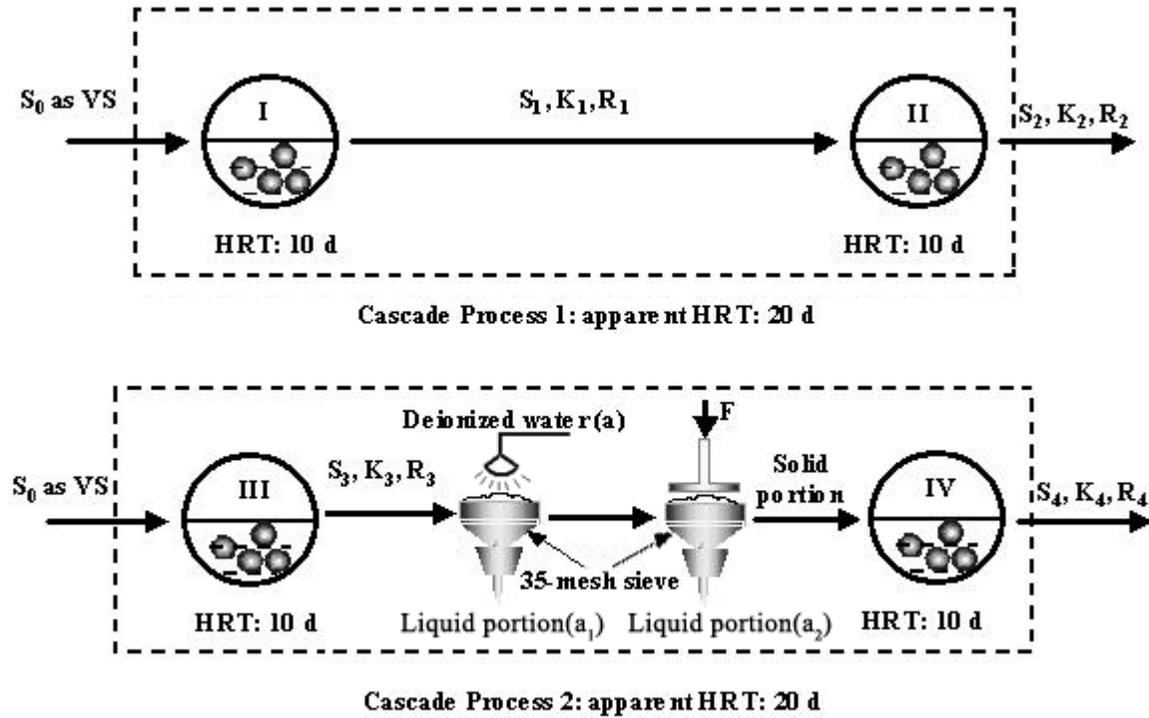
**Fig. 1. Process configurations of the continuous experiment.**  $a$  (g): the weight of the deionized water added daily, 50g;  $a_1$  (g): the weight of the liquid leached when flushing;  $a_2$  (g): the weight of the liquid leached by juice presser,  $a_1 + a_2 = 50$ g;  $S$  (g-VS/L): VS concentration in each stream;  $K$  (/d): the hydrolysis rate constant of each fermenter;  $R$ : the VA increasing ratios;  $P$ : juice presser.
