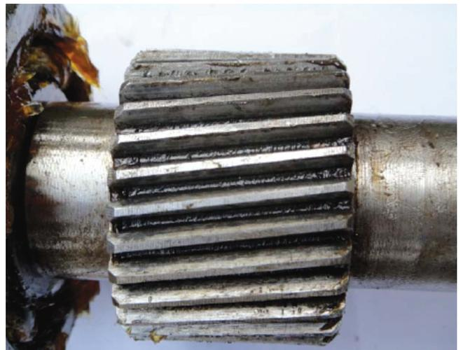
Figure 3. The pitting faulty gear
