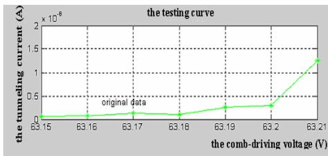
Figure8 testing data about the tunneling current and the comb-driving voltage
