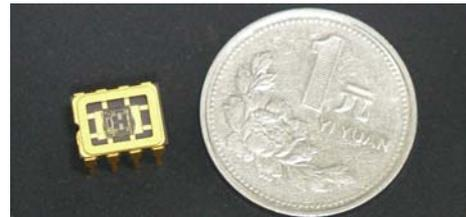
Figure7 the sealed chip of the magnetometer
