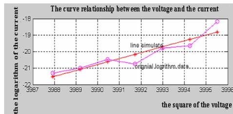
Figure9 relationships between the logarithm of the tunneling current and the square of the comb-driving voltage
