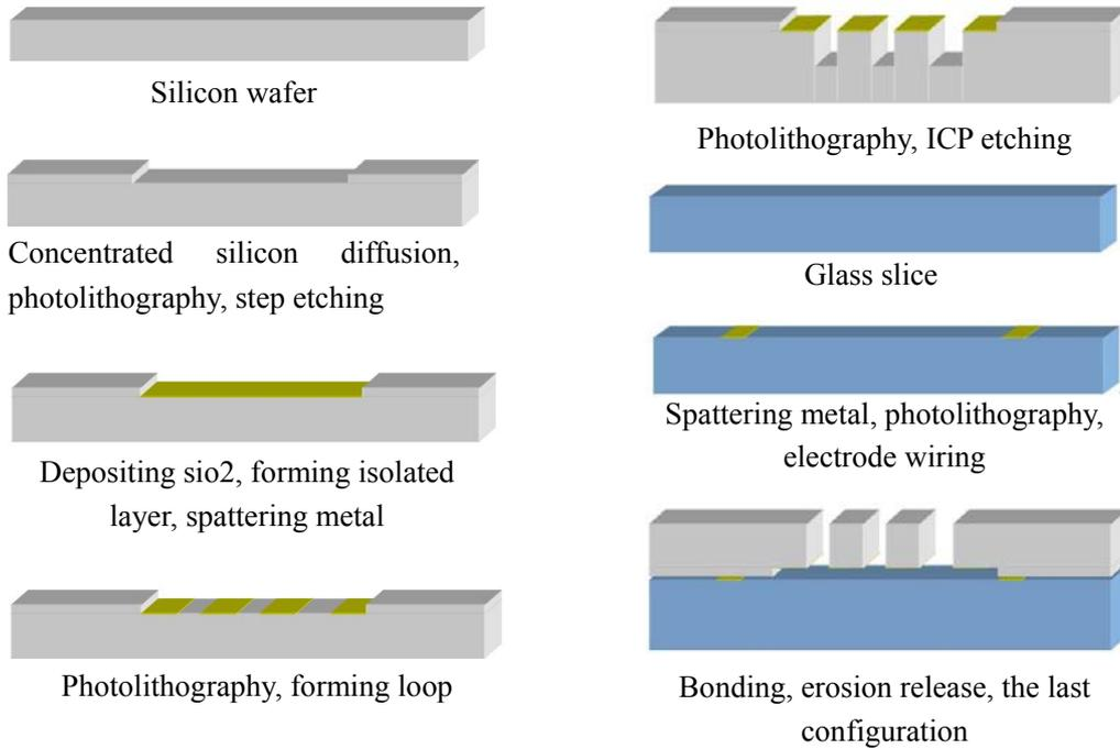
Figure6 Machining Technology
