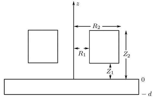
Fig. 1. The sketch of the cross section of coil in cylindrical coordinates, the small coil with the number of turns  $P = 528$ , the inner radius  $R_1$  of 1 mm, the outer radius  $R_2$  of 2.5 mm and the height of 1.0 mm, is mounted on a superconducting film. The film-coil distance  $Z_1$  is 0.25 mm. The thickness  $d$  of the film is 700 nm.
