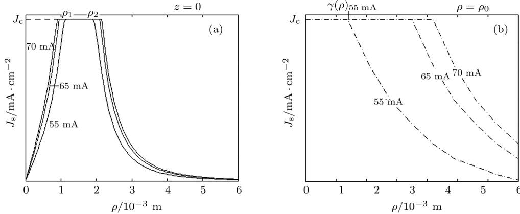
Fig. 4. The distribution of  $J_s$  in the critical state for different driving currents ( $I_0 = 55, 65, 70$  mA): (a) at  $z = 0$  plane; (b)  $\rho = \rho_0$  camber.
