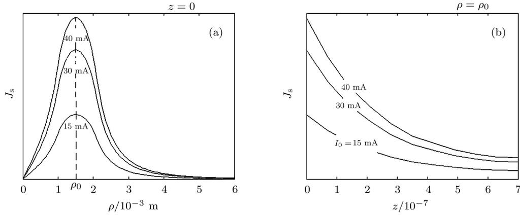
**Fig. 2.** The distribution of  $J_s$  in the Meissner state for different driving currents ( $I_0 = 15, 30, 40$  mA): (a) at  $z = 0$  plane,  $J_s$  value is maximal at  $\rho = \rho_0$  in the horizontal direction; (b)  $\rho = \rho_0$  camber,  $J_s$  value decreases along  $z$  axis.
